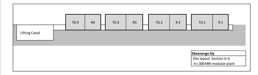
Modules can be lifted 10-20 m up by using a lifting canal
