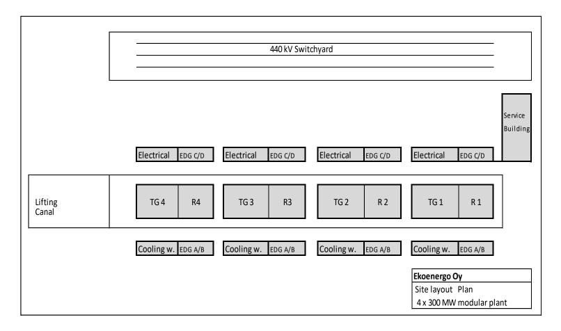
Reactor module: 40 m wide, 60 m long Turbine module: 40 m wide, 80 m long
