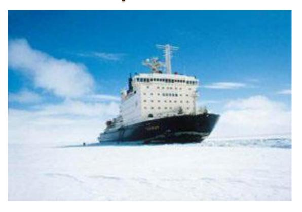
Nuclear Icebreaker (Wärtsilä Helsinki Shipyard) Ordered 1987 Launched 1989 KLT-40 reactor and 2 x 18 MW steam turbines
