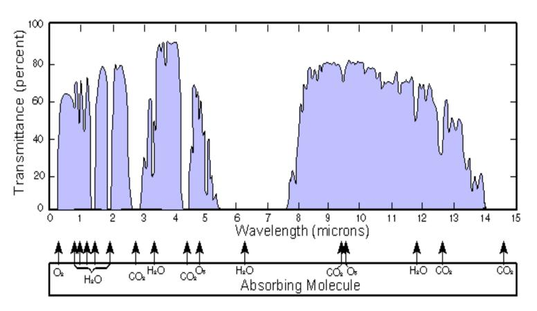
Transmittance of IR radiation depends on CO2 content and wavelength
